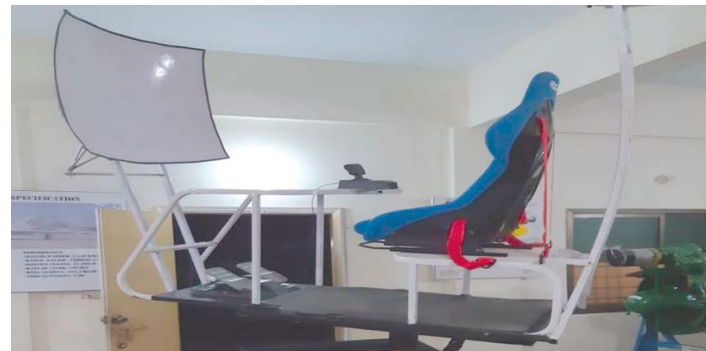
Pakistan's first indigenously developed 4-DOF Motion-Actuated Flight Simulator for Real-Time Testing of Flight Control Computers
